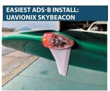
For the second year in a row the editor's choice for a budget ADS-B Out solution goes to uAvionix and the skyBeacon wingtip LED position/strobe system with integral
